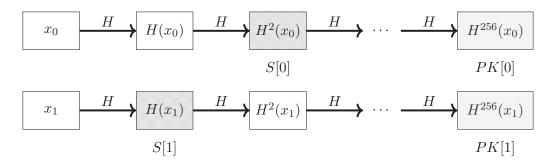
Pictured: A signature over the two-byte message M = [0x02, 0x01], with signature and public key:  $S = [H^2(x_0), H(x_1)], PK = [H^{256}(x_0), H^{256}(x_1)].$
